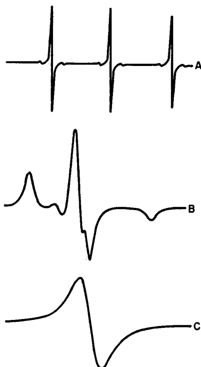
FIGURE 2 Nitroxide spin label spectra illustrating motional and concentration effects. In all three spectra H increases from left to right; A and C are 50 G scans, and B is a 100 G scan. ( A ) Free tumbling of 2,2,6,6-tetramethylpiperidone- N -oxyl (TEMPONE) in water. ( B ) Immobilized spectrum of 12-nitroxide stearate bound to bovine serum albumin. ( C ) Exchange signal of TEMPONE in water.
